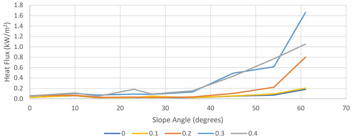
**Figure 2.** The comparison of the slope angle versus the simulated heat flux in STARCCM+ at wind speeds between 0 and 0.4 m/s.
