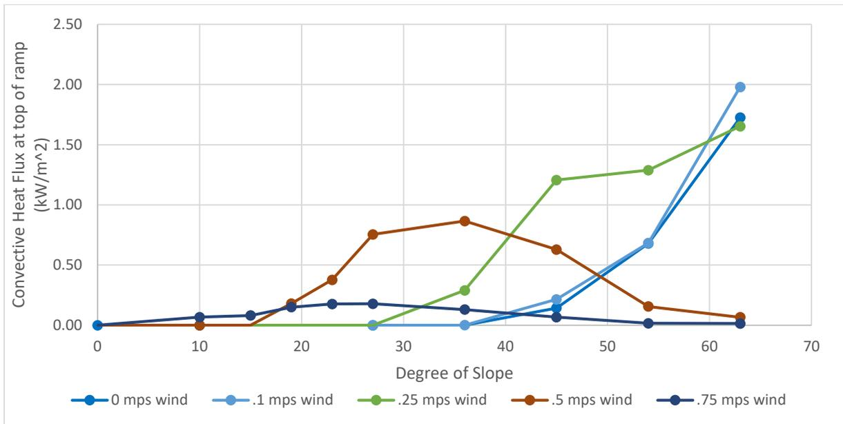
**Figure 5.** The comparison of the slope angle versus the simulated convective heat flux in FDS with a set wind velocity between 0 and 0.75 m/s wind speeds.
