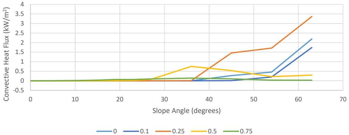
**Figure 4.** The comparison of the slope angle versus the simulated convective heat flux in FDS with dynamic pressures between 0 and 0.75 m/s wind speeds.
