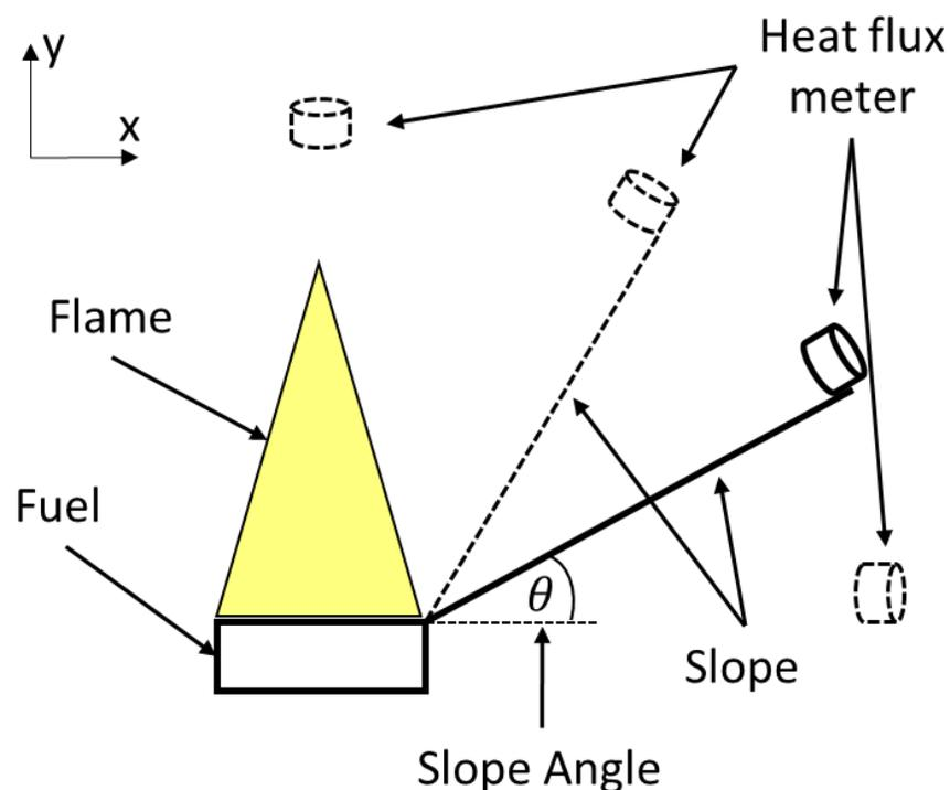
Figure 1. Experimental apparatus showing fuel pan, flame, slope and heat flux sensor placement (from Gallacher, 2016).
