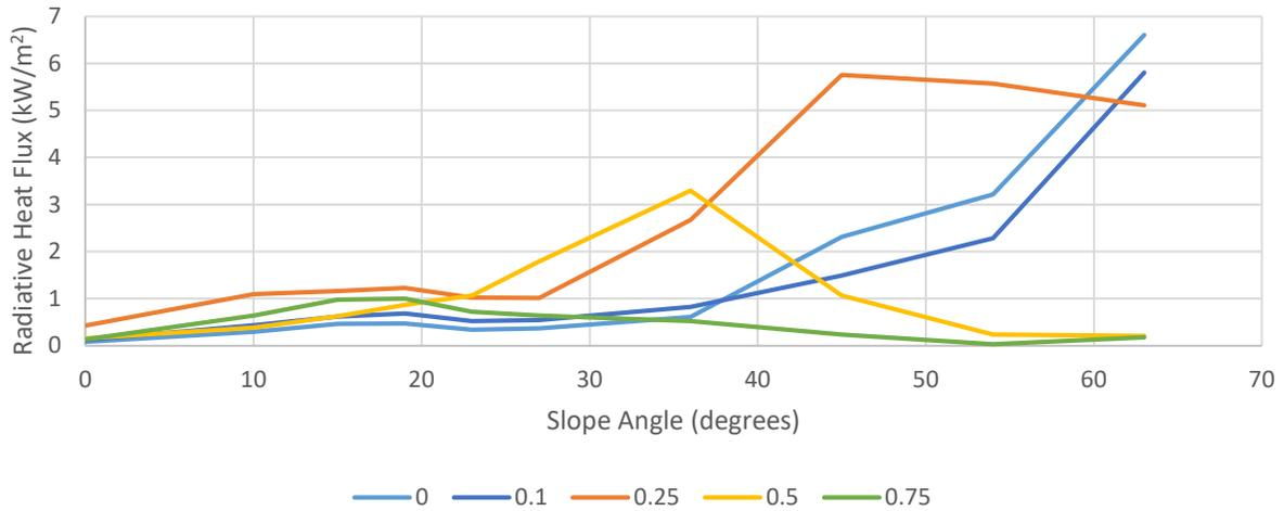
**Figure 6. The comparison of the slope angle versus the simulated radiative heat flux in FDS with dynamic pressures between 0 and 0.75 m/s wind speeds**
