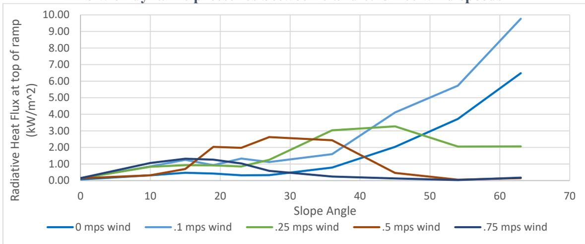
**Figure 7. The comparison of the slope angle versus the simulated radiative heat flux in FDS with a set wind velocity between 0 and 0.75 m/s wind speeds.**
