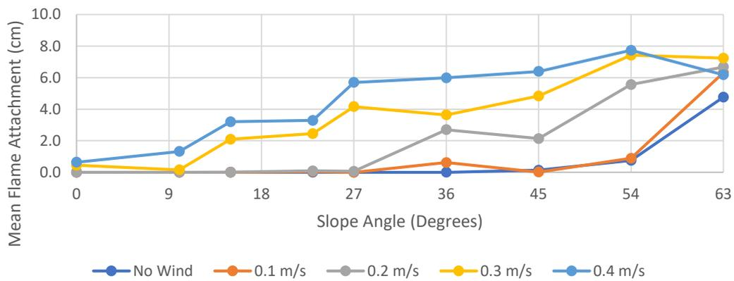
**Figure 3.** The comparison of the slope angle versus the average flame attachment length (cm) in STARCCM+ at wind speeds between 0 and 0.4 m/s
