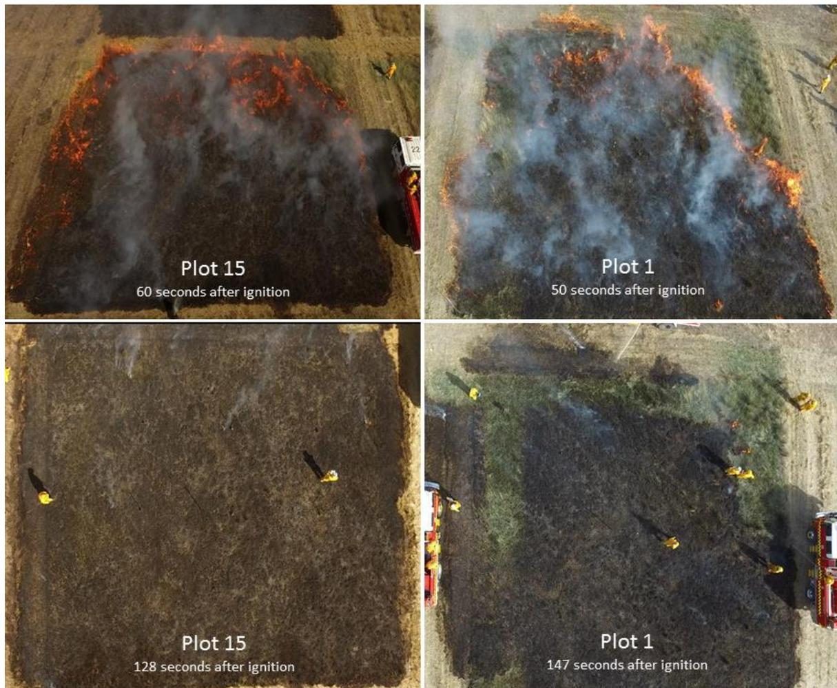
Figure 2 Aerial view of fires reaching the control line and the remaining fuel in the plots with the longest (plot 15, 4 h 16 min) and shortest (plot 1, 36 minutes) time since application.
