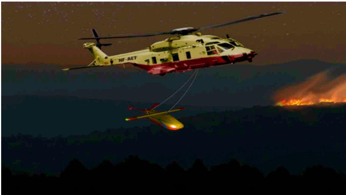
**NitroFirex Autonomous Glider Containers (AGC) dropping their contents with utmost precision in the source of the fire.**
