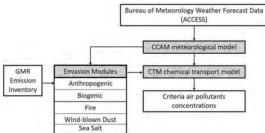
Figure 1: Schematic diagram of the operational CCAM-CTM modelling system
