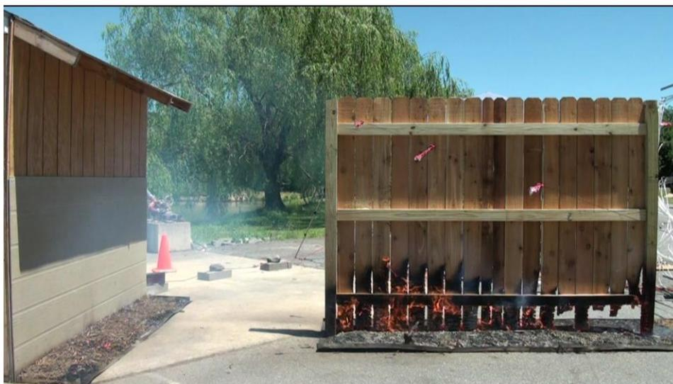
Figure 2: WRC privacy fence with HW mulch, in medium wind, at  $t = 5$  min.
