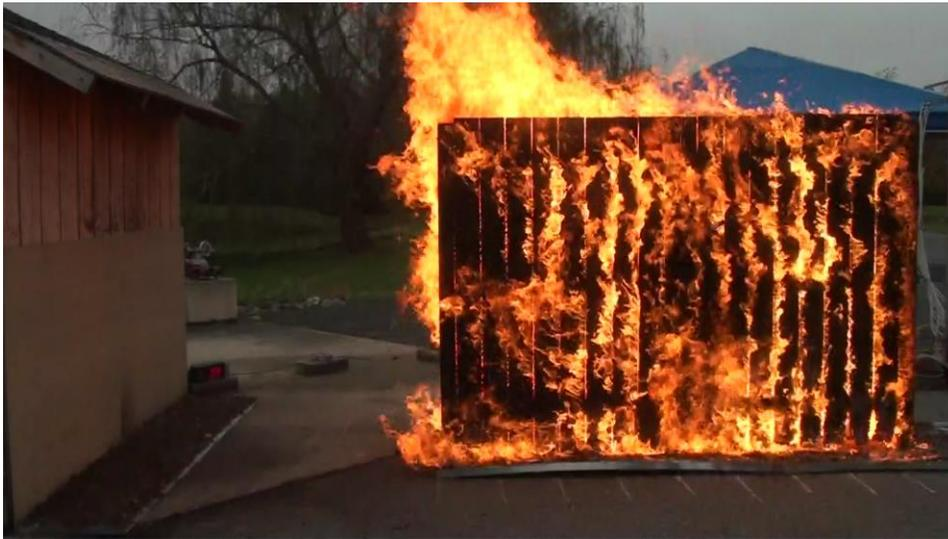
**Figure 3: Parallel WRC privacy fences spaced apart by 20 cm, with HW mulch in low wind, at  $t = 5$  min.**
