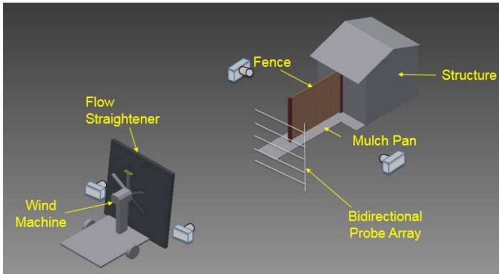
Figure 1: Experimental setup
