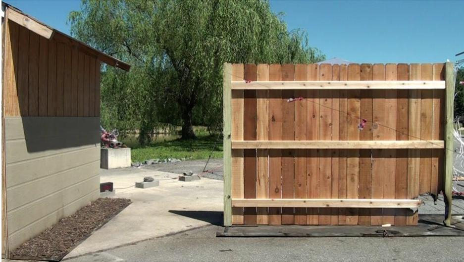
**Figure 4: WRC privacy fence without mulch, in medium wind, at  $t = 30$  min.**
