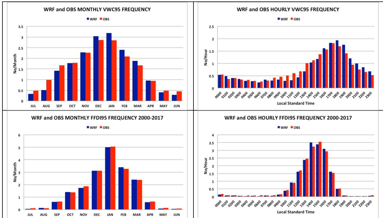
Figure 2. Average frequency distributions by month and by hour of 95<sup>th</sup> percentile highest daily VWC and FFDI events for all 22 locations from the WRF and from AWS observations for the period 2000-2017. NB Times are Local Standard Time.
