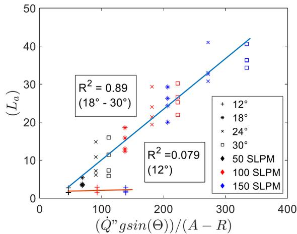
Fig 6. Attachment length vs. key parameters for tests inclined from 12° - 30°. The heat-release rate was varied between 76 – 228 kW for fires with 4 different burner depths.
