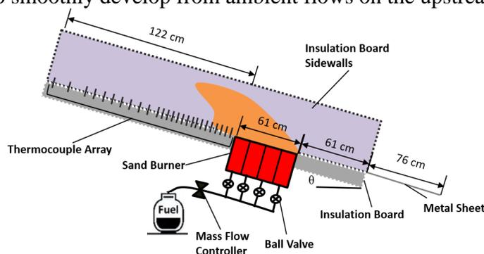
Fig 1. Schematic of the experimental apparatus mounted on a tilt table.
