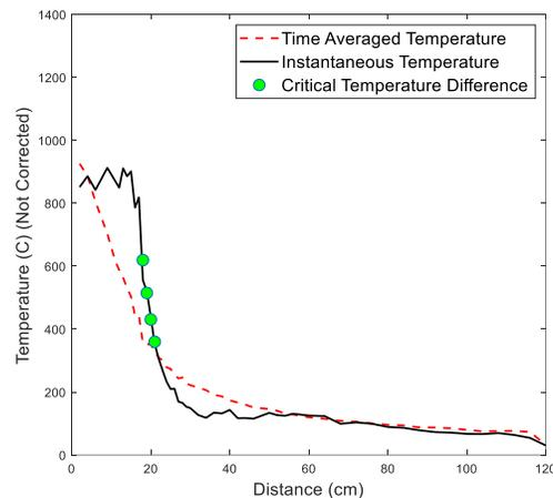
Fig 2. Instantaneous temperature profile (solid line) compared to a time-averaged profile (dashed line) downstream of the burner. Circles indicate the point where a critical temperature difference is observed, based on defined thresholds. Data comes from a 76 kW fire at an incline of 30° with a burner depth of 15 centimeters.
