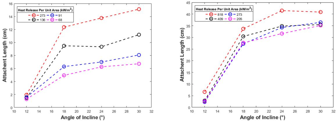
Fig 3. Plots of flame attachment length as a function of the angle of incline for different burner geometries and heat-release rates.
