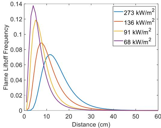
Fig 4. Histograms of flame liftoff length from four different overall heat release rates compared. Data comes from a 76 kW fire at an incline of 30° with four different burner depths.
