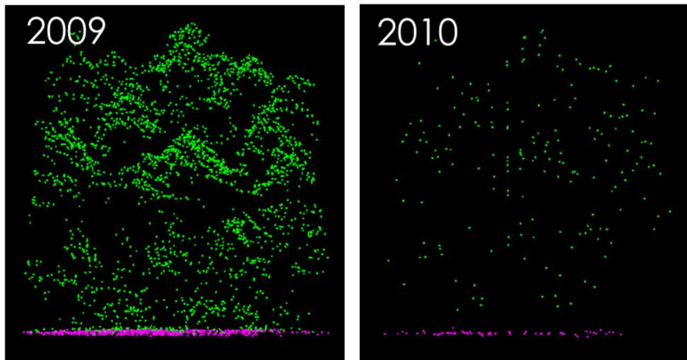
**Figure 1.** Example point clouds of the same plot from both LIDAR dataset: medium pulse density (2009) and low pulse density (2010)
