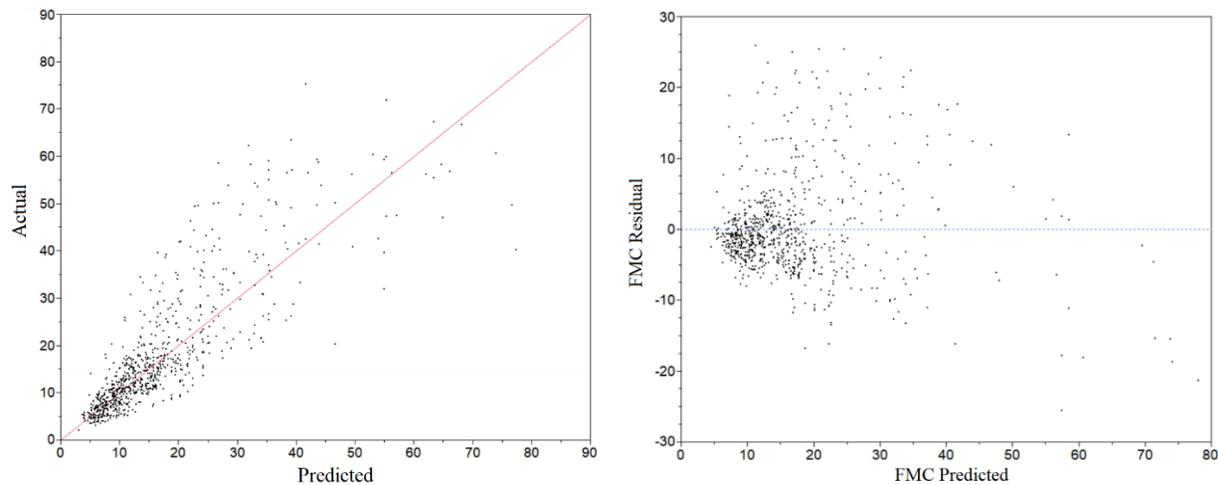
Figure 2 – On the left side, plot of observed fine dead FMC (Actual) versus predicted (using the proposed model). On the right, plot of residuals versus predicted response.
