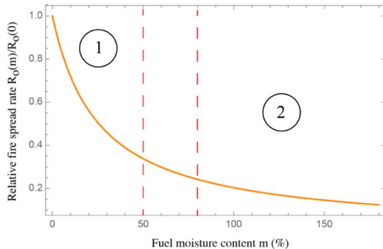
**Figure 1: Theoretical relative fire spread rate ( $R_o(m)/R_o(0)$ ) as a function of moisture content ( $m$ ). Fuel bed: *Eucalyptus Globulus Labill* leaves ( $e = 7.5$  cm;  $S_e = 1.5$ )**
