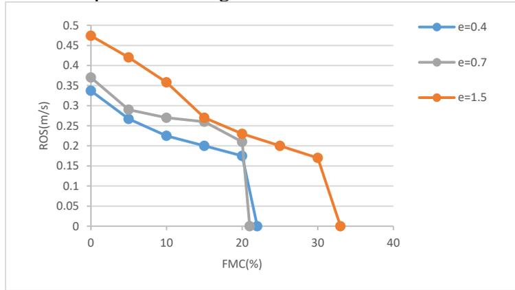
**Figure 4: The rate of spread variation as a function of fuel moisture contents (m) for three different fuel bed depth (40cm ,70cm, 150cm) Fuel bed: grassland**
