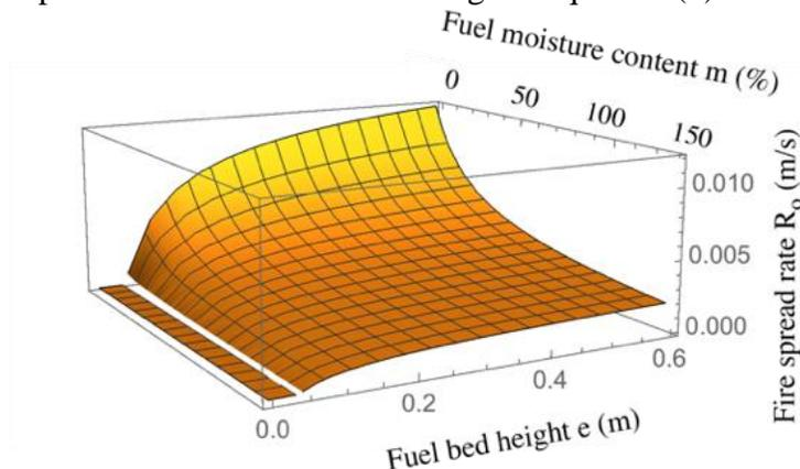
**Figure 3: Theoretical rate of spread variation  $R_o$  as a function of fuel bed depth ( $e$ ) and fuel moisture contents ( $m$ ). Fuel bed: Eucalyptus Globulus ( $S_e = 1.5$ )**
